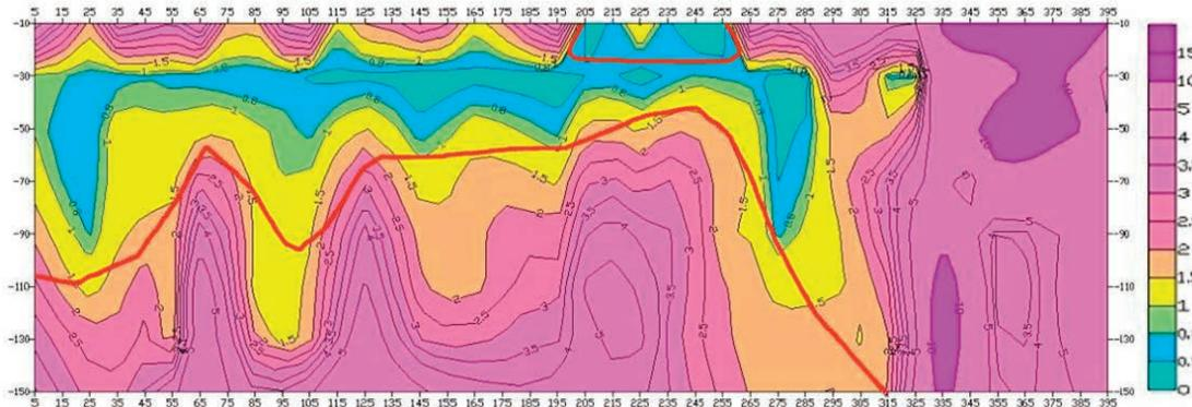
**Fig. 2** Apparent resistivity section of the floor of track tunnel for E3206 work face.
