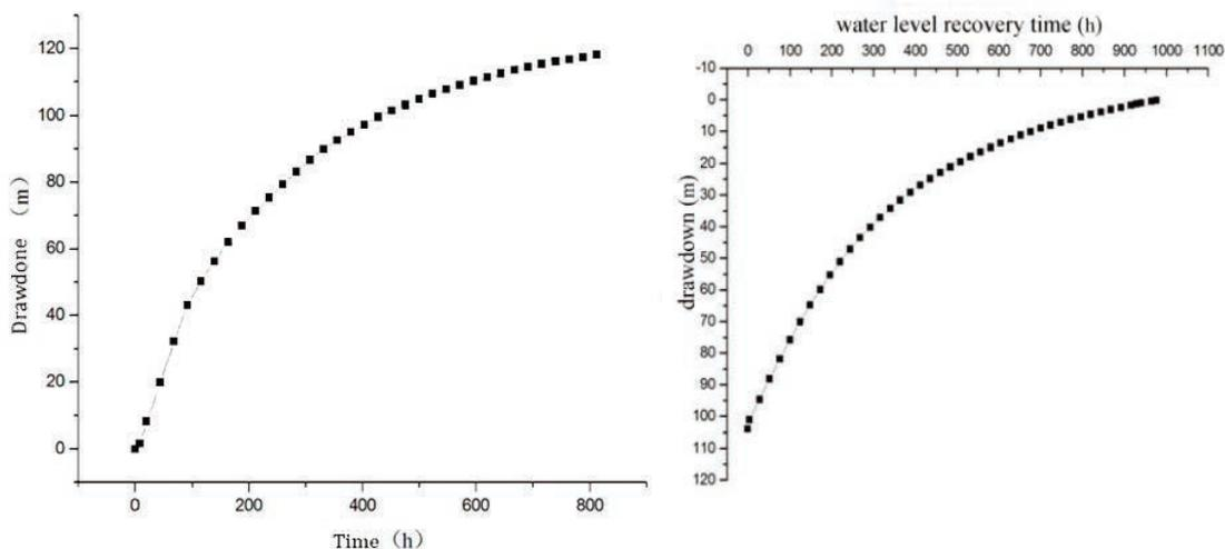
**Fig. 3** Curves of drawdown-time in S5 during the dewatering and recovery tests. left: dewatering; right: recovery.
