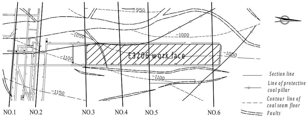
**Fig. 4** Distribution of the six section lines in E3206 work face
