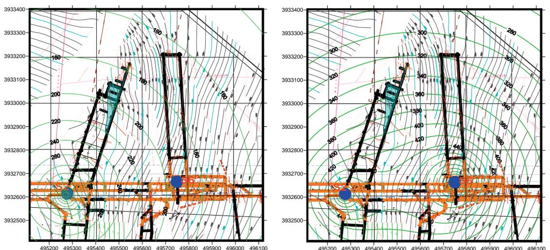
**Fig. 5** left: Contour map of drawdown before drainage in E2306 work face; right: Contour map of forecasting drawdown after 60 days of drainage
