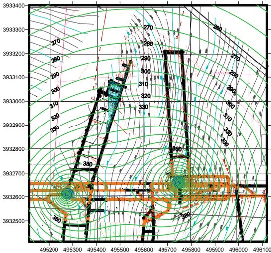
**Fig. 6** Contour map of drawdown after drainage and before mining in E2306 work face.
