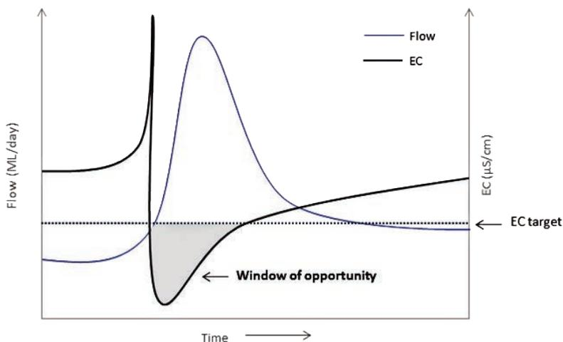
**Fig. 3** Calculation of Total Allowable Discharge is based on the repetitive decrease in salinity as flow increases.
