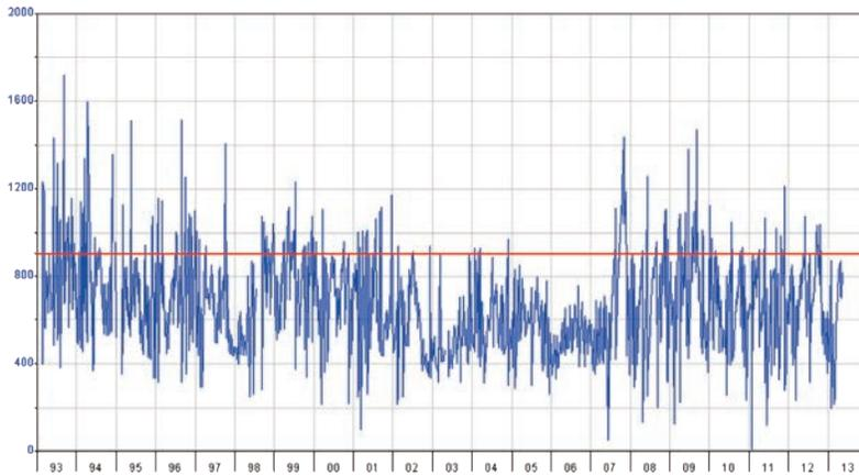
**Fig. 2** Mean monthly Electrical Conductivity at Singleton 1993 – 2013. Red line is the salinity target.
