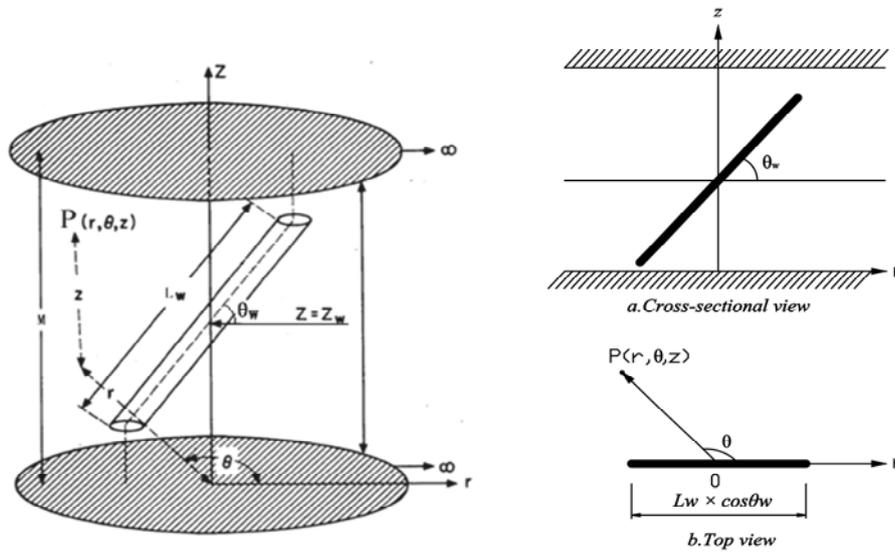
Fig. 1 Schematic slanted well in confined aquifer
