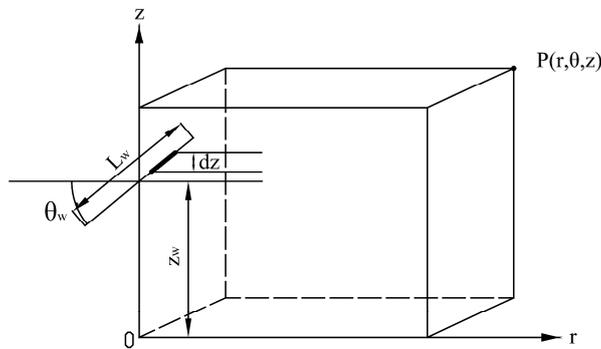
**Fig. 3** Location infinite space aquifer inclined line sink and observation points
