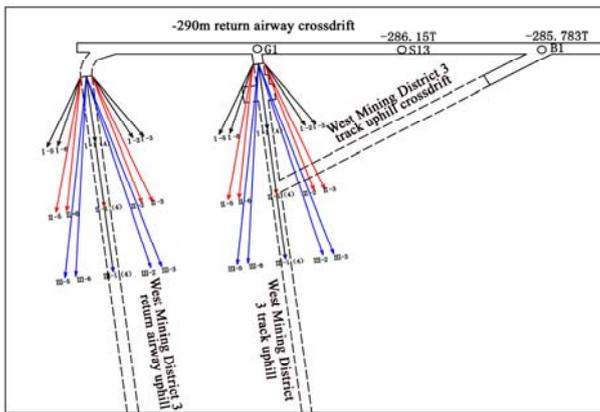
*Fig. 1* Layout plan of drill holes for advanced curtain grouting
