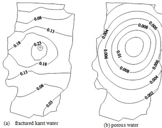
**Fig.3** Contour map showing the spatial distribution of the additional drawdown in the Quaternary porous aquifer and the Ordovician fractured karst aquifer at day 1095
