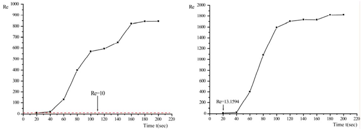
Fig. 5  $R_e$ -curve of No.1 fault water inrush ( $P_w=3, 5$  MPa)
