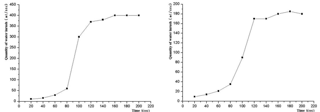
**Fig. 10**  $Q$ -curve of No.3 fault water inrush ( $P_w=3, 5$  MPa)
