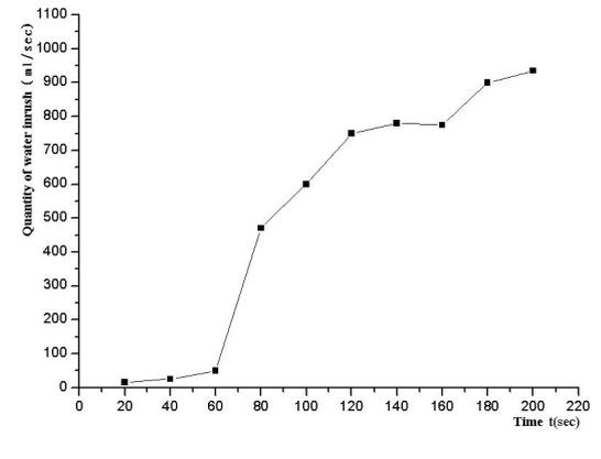
**Fig. 9** *Q*-curve of No.2 fault water inrush ( $P_w=3, 5$  MPa)
