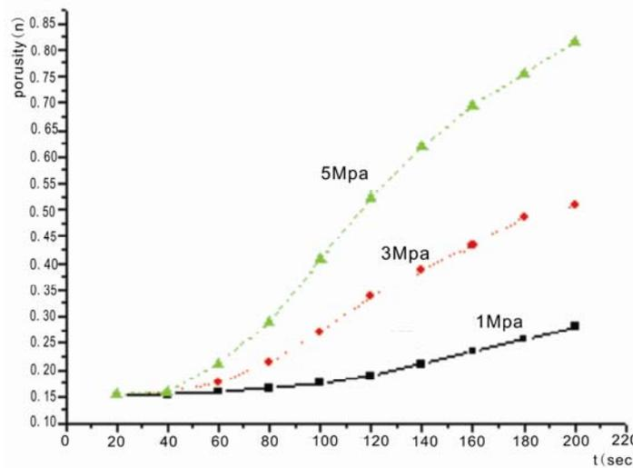
Fig. 13  $n$ -curve of No.3 fault water inrush under different pressure
