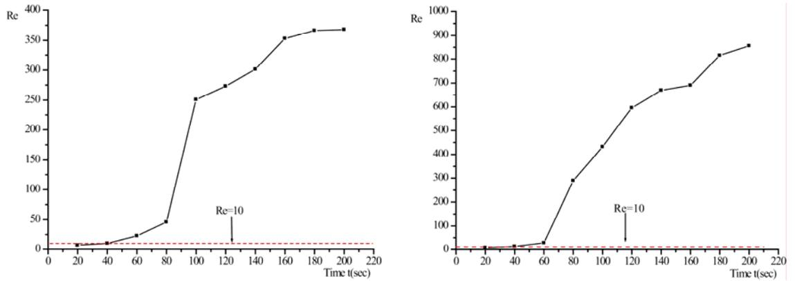
Fig. 6  $R_e$ -curve of No.2 fault water inrush ( $P_w=3, 5$  MPa)
