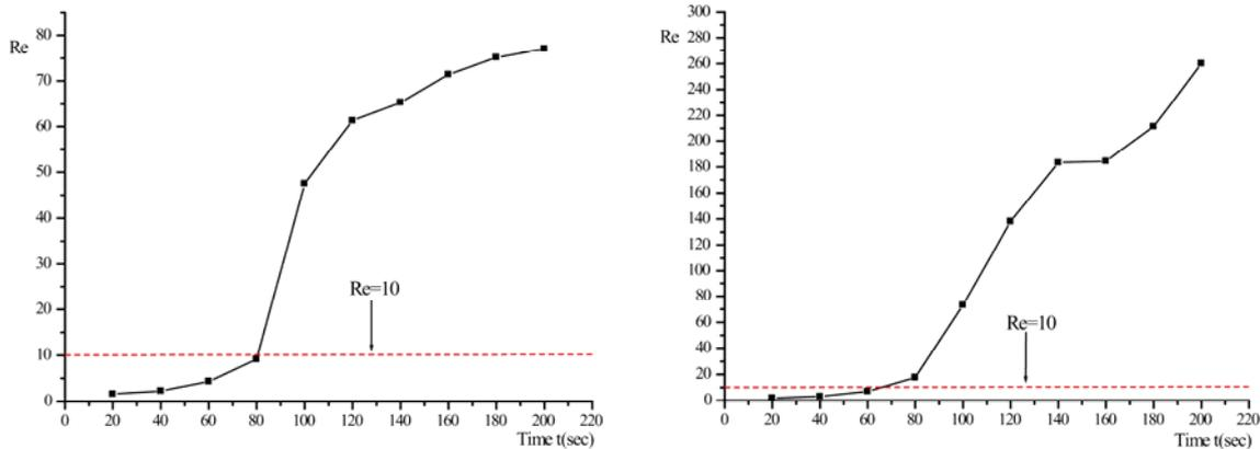
Fig. 7  $R_e$ -curve of No.3 fault water inrush ( $P_w=3, 5$  MPa)
