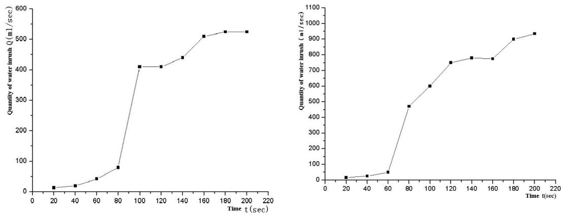
**Fig. 9**  $Q$ -curve of No.2 fault water inrush ( $P_w=3, 5$  MPa)
