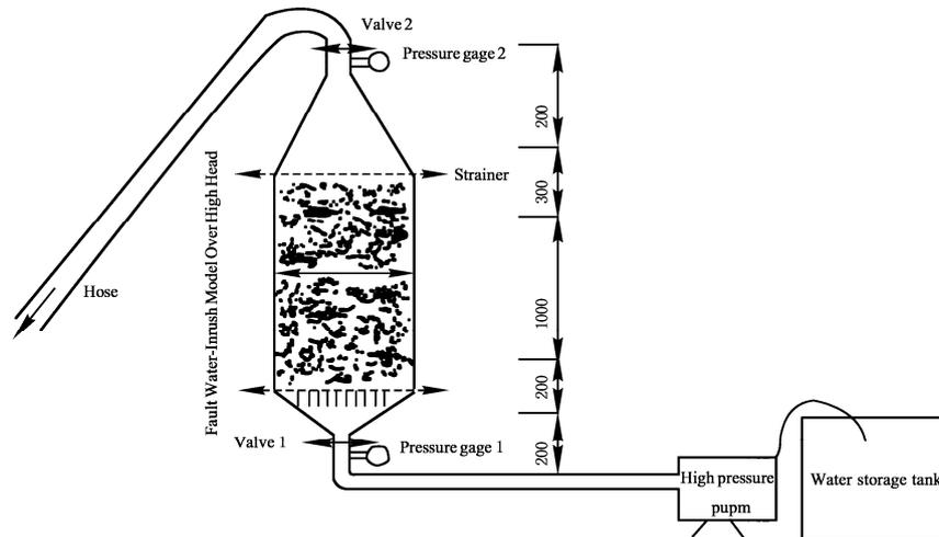
Fig. 3 The sketch of fault water-inrush model over high head
