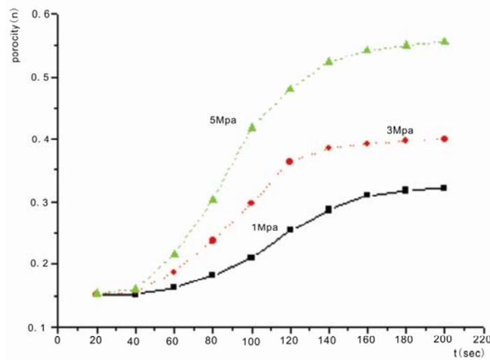
Fig. 12  $n$ -curve of No.2 fault water inrush under different pressure
