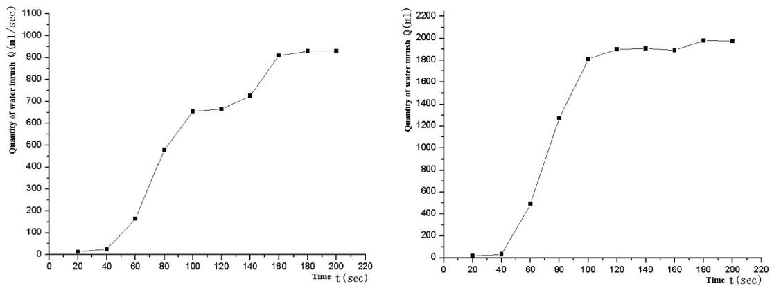
**Fig.8**  $Q$ -curve of No.1 fault water inrush ( $P_w=3, 5$  MPa)
