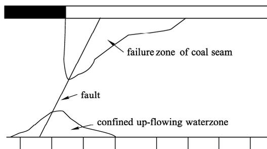
Fig. 4 The sketch of Mining fault water-inrush
