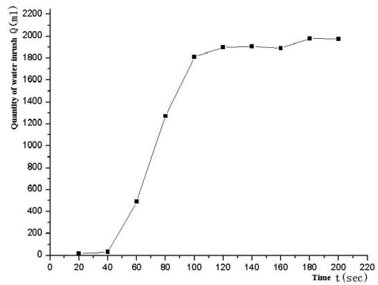
**Fig.8** *Q*-curve of No.1 fault water inrush ( $P_w=3, 5$  MPa)
