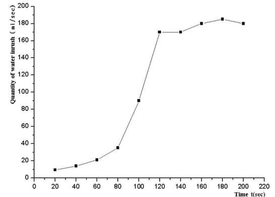
**Fig. 10** *Q*-curve of No.3 fault water inrush ( $P_w=3, 5$  MPa)
