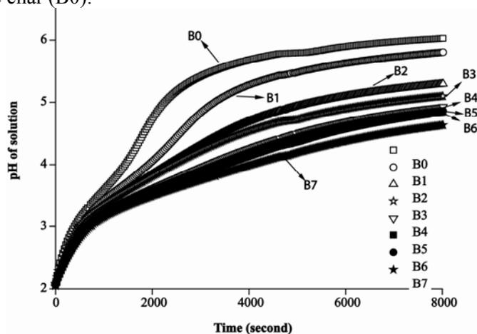
Fig. 4 The neutralization ability of manganese-coated bone char
