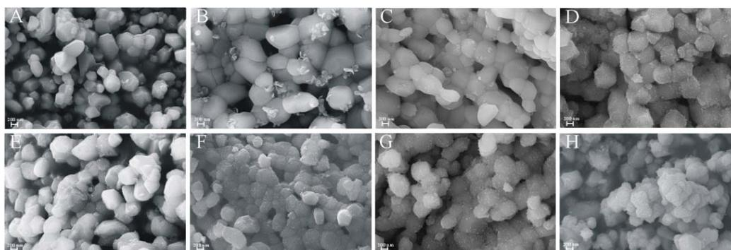
*Fig.2 SEM micrographs of the particles of the manganese-coated bone char (A. B0, B. B1, C. B2, D. B3, E. B4, F. B5, G. B6, H. B7. The detailed numbers are given in table 1. )*
