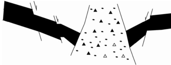
Fig. 2 Development of small fault in the surrounding rock of karstic collapse column
