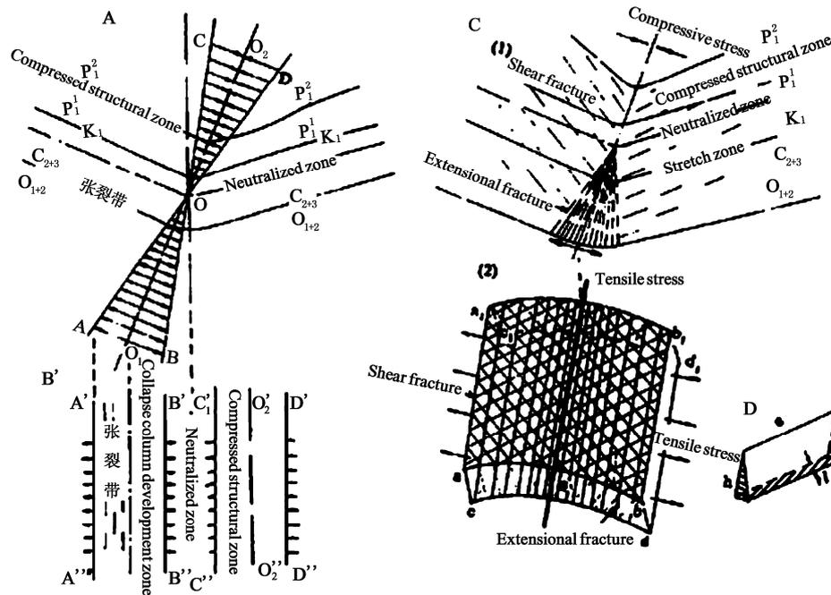
Fig. 3 Schematic Diagram of Relation between Chenji Syncline and Limestone Karst
