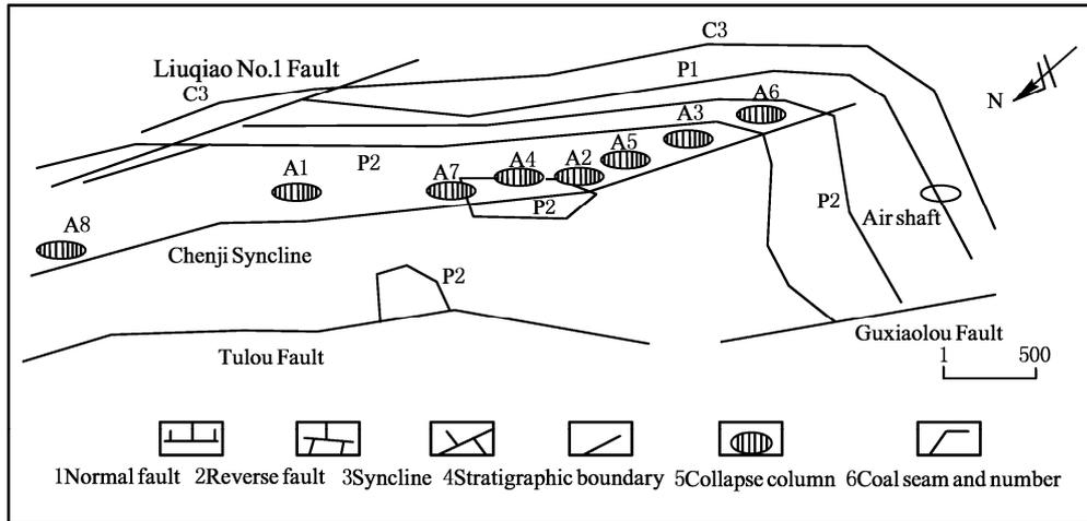
Fig. 1 Layout of Karstic collapse columns of Liuqiao No.1 Coal Mine
