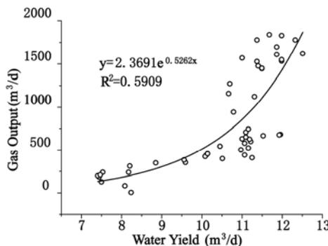
Fig. 4 The relationship between gas output and water yield by well B07
