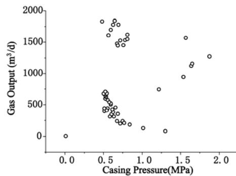
Fig. 3 The relationship between gas output and casing pressure by well B07
