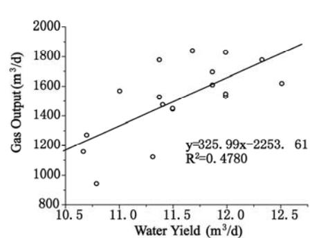
*Fig. 6 The relationship between gas output and water yield by well B07 in the late*
