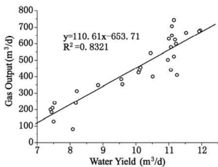
*Fig. 5 The relationship between gas output and water yield by well B07 in the middle*
