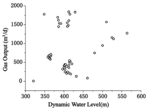
Fig. 2 The relationship between gas output and dynamic water level by well B07
