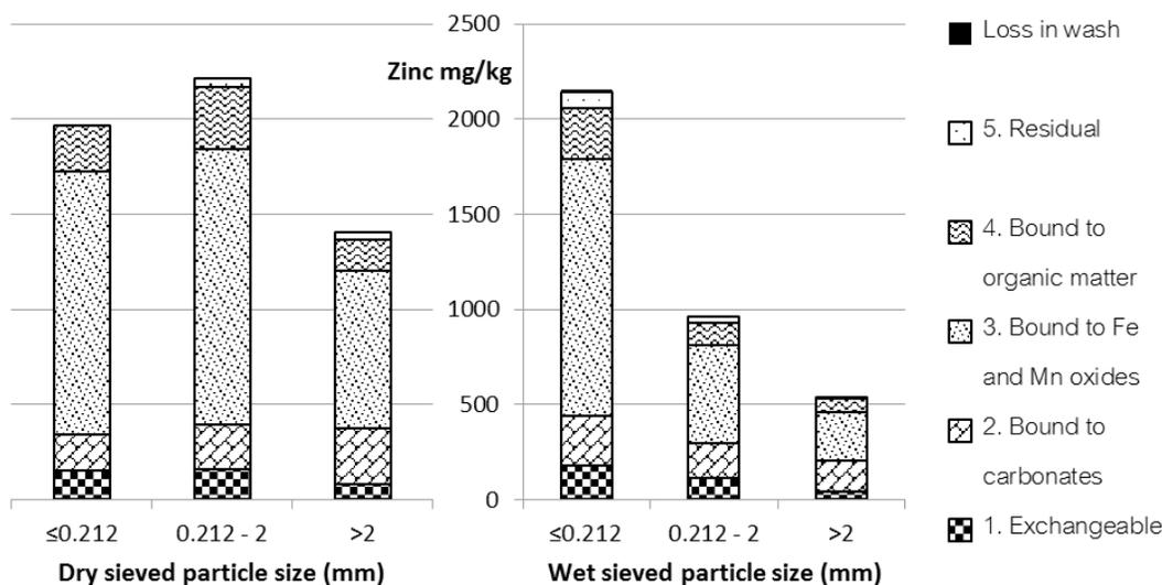
Figure 4 Zinc concentrations in sieved substrate samples
