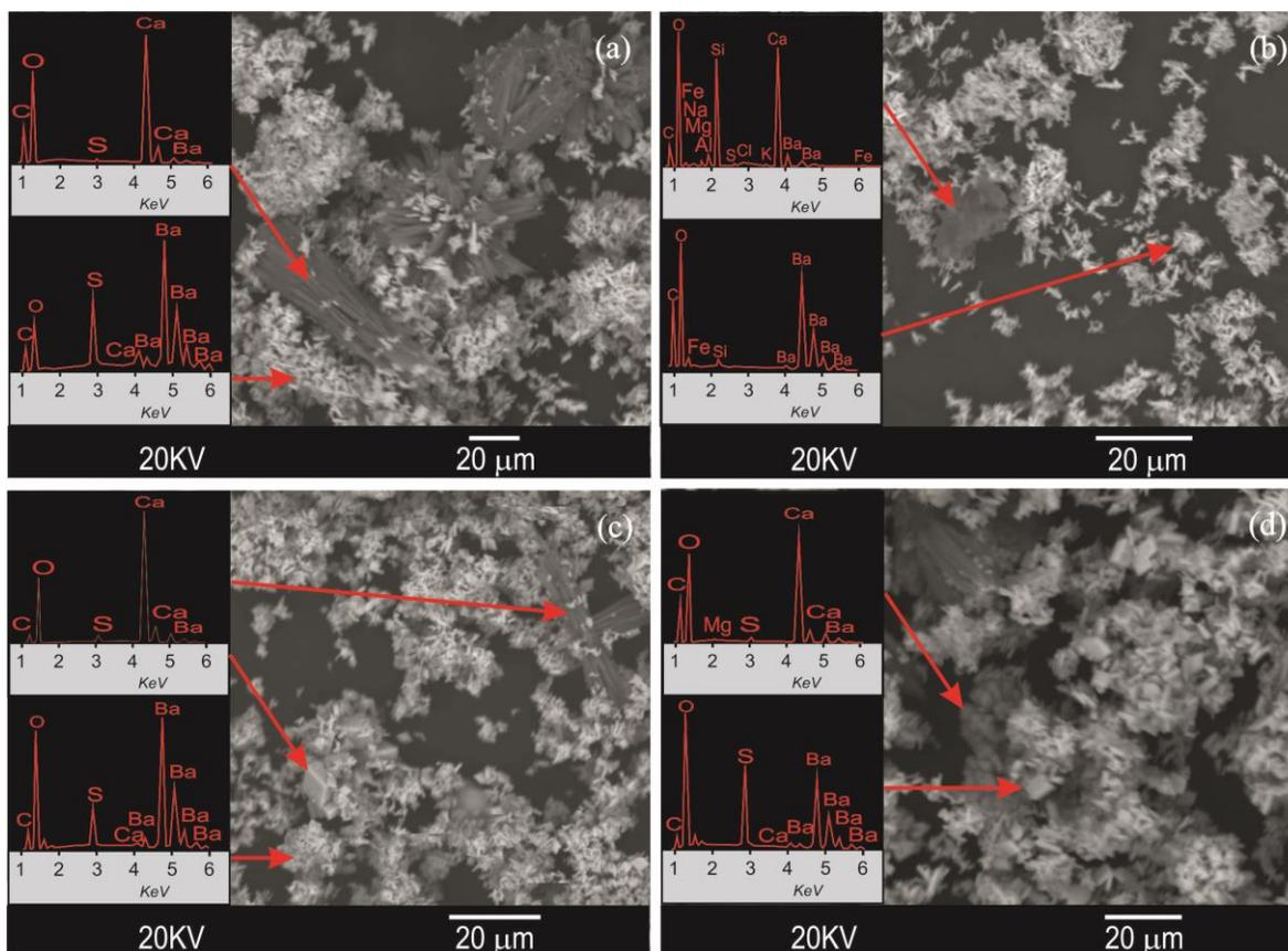
**Figure 3** SEM images of (a) top sample: fibrous aggregates of CaCO<sub>3</sub>, acicular BaSO<sub>4</sub>, (b) amorphous precipitation and BaCO<sub>3</sub>; (c) middle sample: fibrous and rhombohedral crystals of CaCO<sub>3</sub> and acicular BaSO<sub>4</sub> (d) globular CaCO<sub>3</sub> and orthorhombic BaSO<sub>4</sub>.
