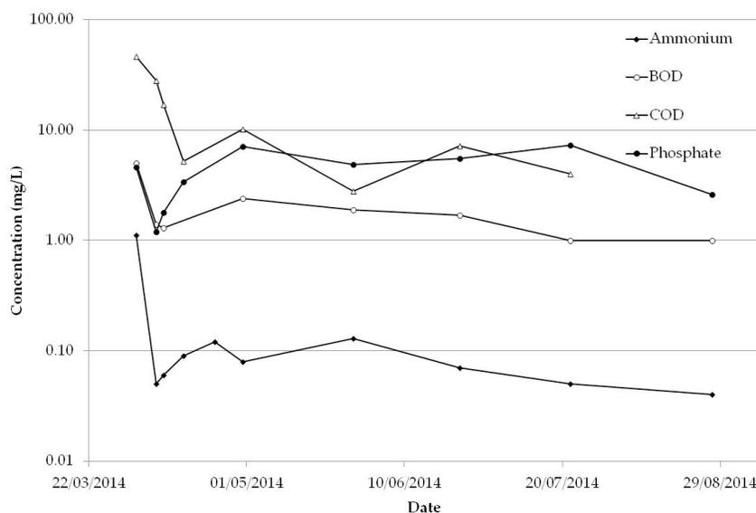
Figure 5 Concentrations of BOD, COD, NH<sub>4</sub> and PO<sub>4</sub> in the Coledale Beck downstream of the treatment system following commissioning in March 2014
