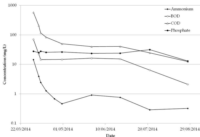
**Figure 4** Concentrations of BOD, COD, NH<sub>4</sub> and PO<sub>4</sub> in the final effluent from the treatment system following commissioning in March 2014
