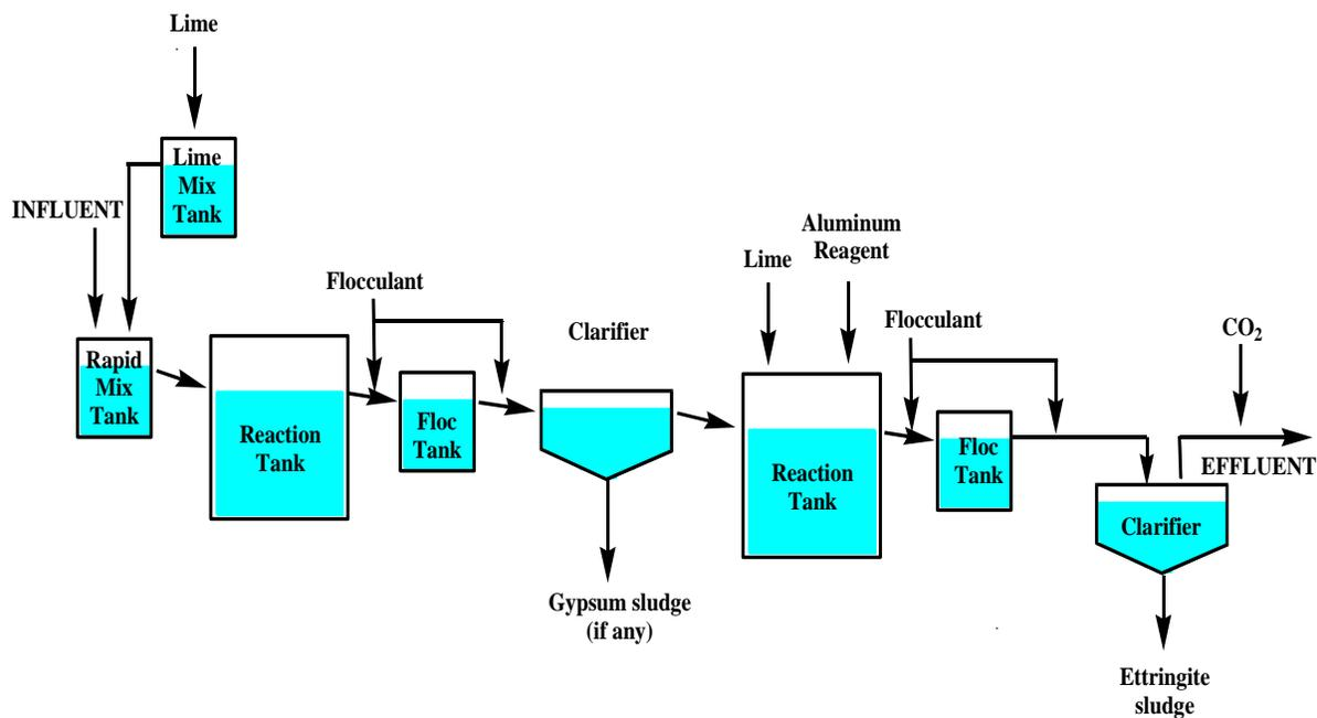
Figure 2 Schematic of CESR sulfate removal process
