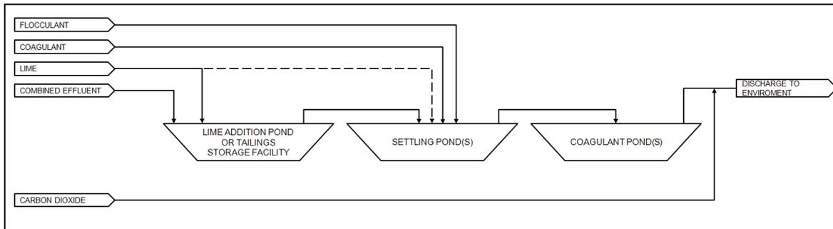
Figure 2 Base metal subsector effluent treatment model
