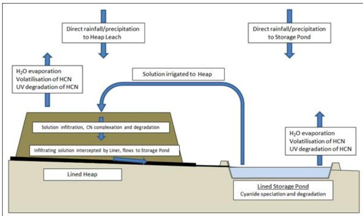
**Figure 1** : Conceptual model of the system
