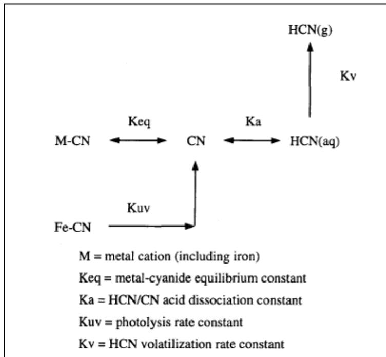
**Figure 2:** Routes to Hydrogen Cyanide volatilization (from Botz and Mudder, 2000)
