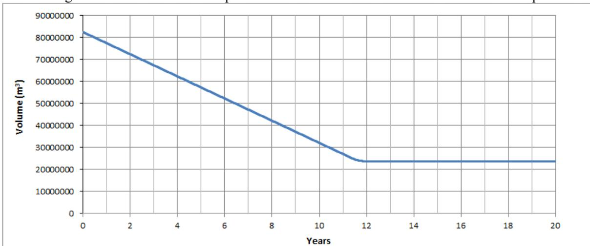
Figure 3. As the degree of saturation the heap decreases, the rate of seepage also decreases, due to the reduction in the effective hydraulic conductivity. The moisture content within the heap steadily decreases to a point at which the moisture content reaches the specific retention value (assumed to be 10%) such that the net moisture entering the system as recharge is effectively equivalent to the rate of seepage discharging from the base of the heap.
