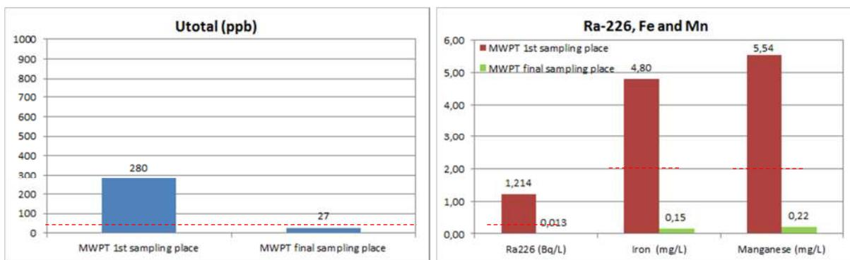
Figure 3 Mine water PTS efficiency by comparing initial and final concentrations along treatment path (medium values in the first semester 2015) in Urgeriça mine - Shaft4
