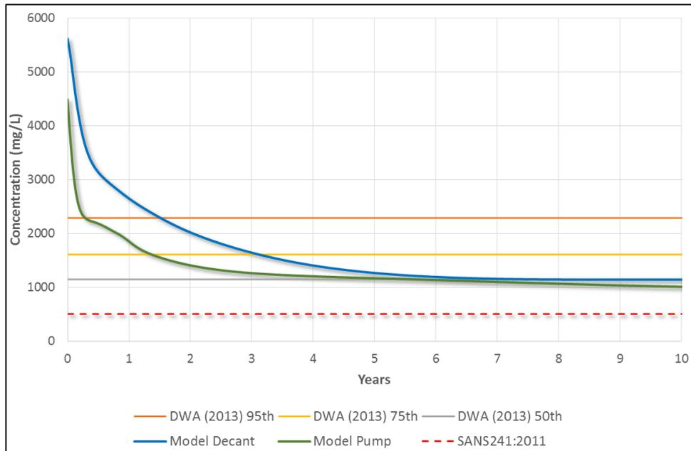
**Figure 7** Calculated sulphate development for various scenarios
