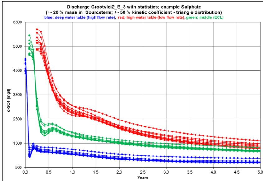
Figure 8 Uncertainty analysis - calculated sulphate development
