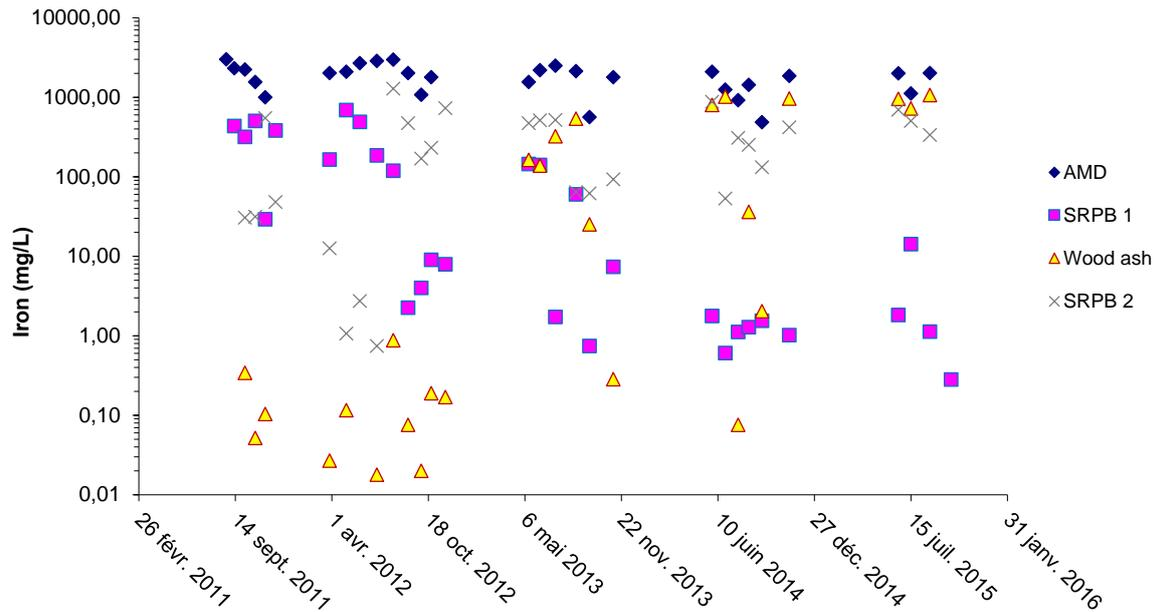
**Figure 4** Iron concentrations in each of the three-unit the passive treatment system constructed on Lorraine mine site, Quebec, Canada.
