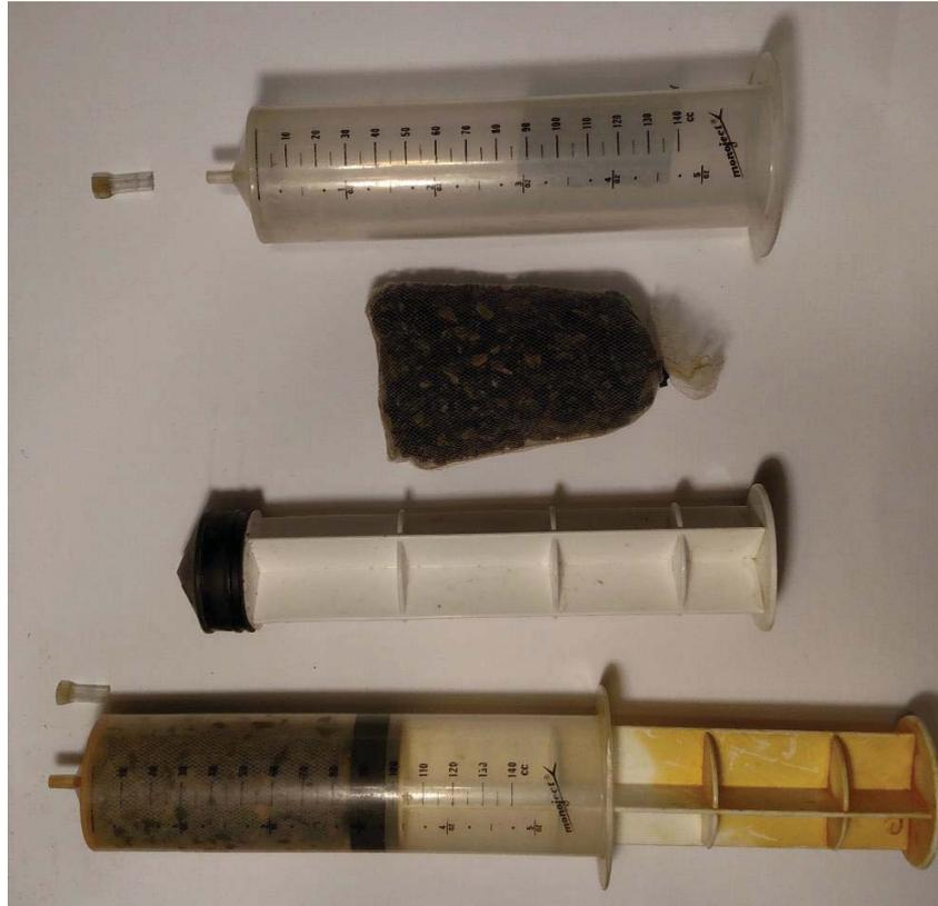
**Figure 1** The standard composition of an Alkast is a 140 mL syringe, a mesh bag with material, and an airtight cap.
