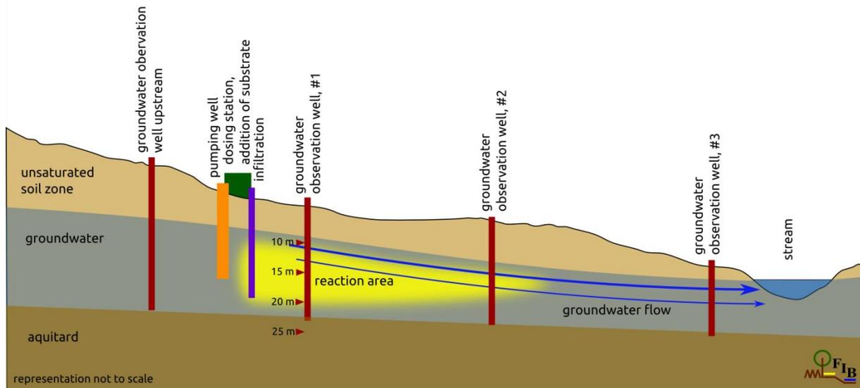
**Figure 1** Vertical section through the test area.
