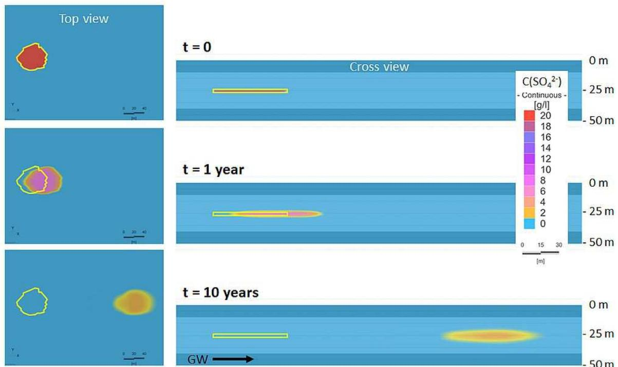
**Figure 5** Fate of tracer solution ( $SO_4^{2-}$  in g/L) from an abandoned mine site in horizontal (top view) and vertical (cross view) direction caused by groundwater (GW) induced dilution (non-reactive species transport).
