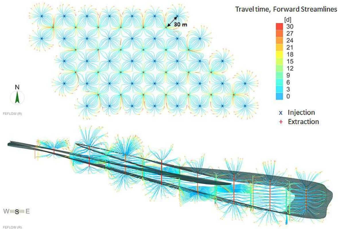
**Figure 2** Optimization of wellfield design for a mineralized rollfront; lixiviant streamlines within a 5-spot well pattern as top view (upper image) and 3D view within the rollfront (lower image). Streamline color is indicative of travelling time (cf. legend).
