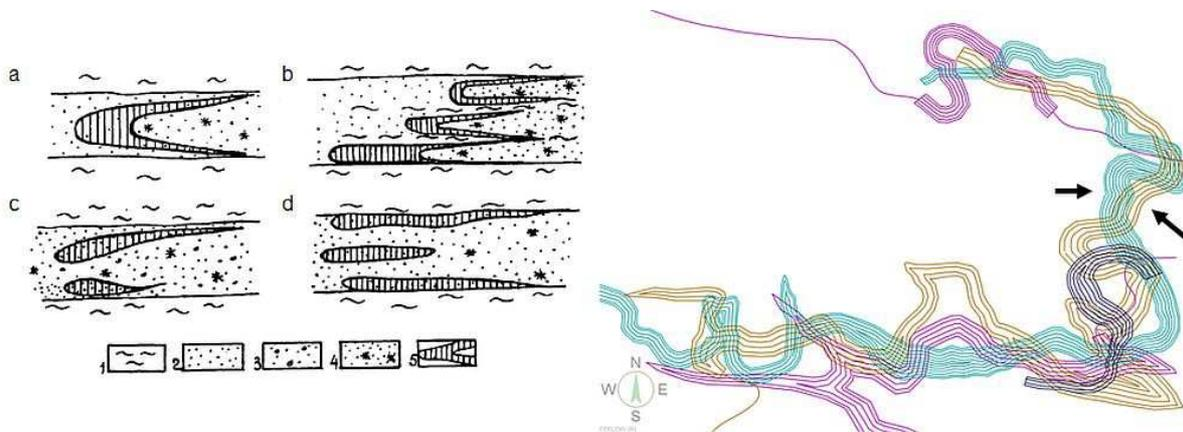
**Figure 1** (Left) Morphology of roll-type deposits: a) simple roll-type deposit, b) series of simple rolls within aquifer with zones of reduced permeability, c) stratiform deposits with no roll, d) lenticular deposits at several levels: 1 - clay, 2 - sand, 3 - gravel, 4 - limonitizations, 5 - ore deposit (modified after IAEA 2001), (Right) Map of multilevel rollfronts in aquifers with different groundwater flow directions.
