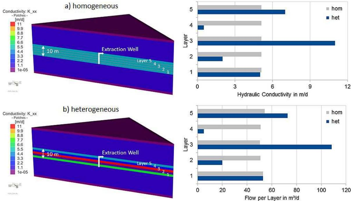
**Figure 3** (Left) 3D model design of a single extraction well (10 m screen) embedded within a (a) homogeneous and (b) heterogeneous aquifer hydraulic conductivity. (Right) Hydraulic conductivity (m/d) and flow rates (m<sup>3</sup>/d) per layer along filter screen for homogeneous (hom) and heterogeneous (het) model.
