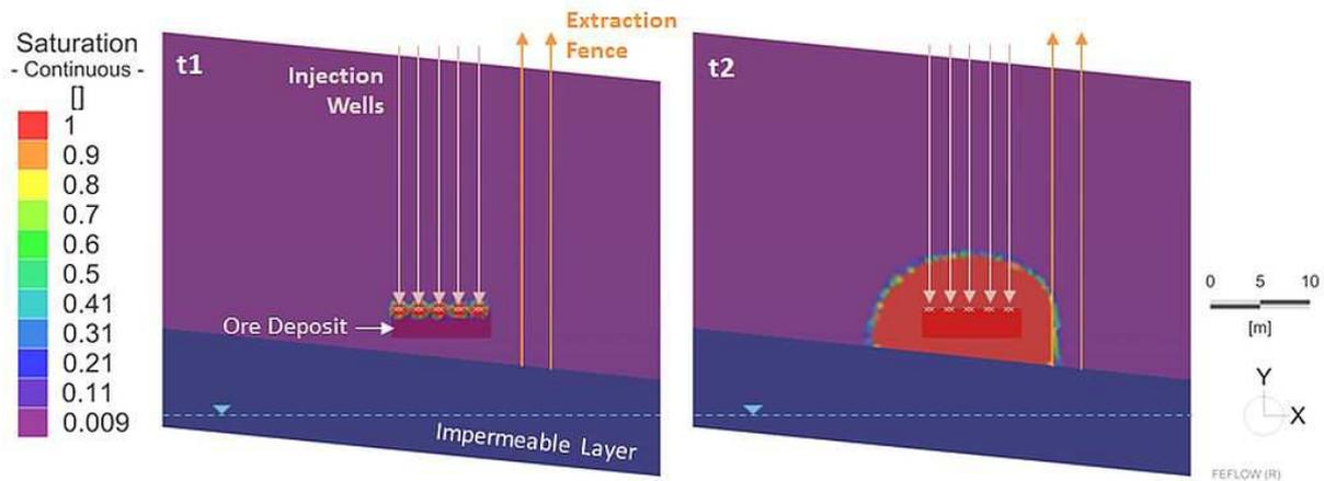
**Figure 4** ISR application within the vadose zone; gravity-driven saturation of the ore deposit and adjacent area for two different time steps  $t_1$  (shortly after startup) and  $t_2$  (reaching extraction).
