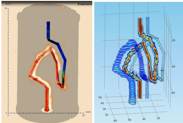
**Fig. 1, left:** Snapshot of a visualized fluid transport inside a tube embedded in a cement core by means of GeoPET; **right:** From right to left: extracted absolute value of  $v(x,y,z)$  and extracted effective porosity  $n(x,y,z)$ ; simulated  $c(x,y,z,t)$  as obtained from a model with an unstructured grid. The observed and modelled transport processes agree well. The 3D velocity field extraction from experimental observations is therewith validated.
