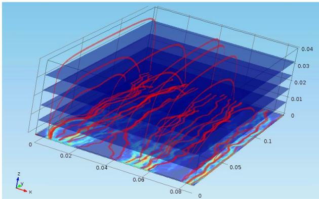
**Fig. 2:** Simulated velocity distribution (rainbow colour) and flow lines (red lines) inside a heterogeneous fracture (bottom) and adjacent porous calciferous sandstone (block above fracture): Outlook: Effective fracture velocities extracted from flow monitoring in fractured cores will be used in a 3D reactive transport model for estimating e.g. the effect of porosity/permeability change due to calcite dissolution and gypsum precipitation.
