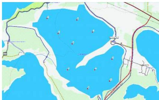
**Figure 1:** proposed pH network for the pit mine lake Partwitz
