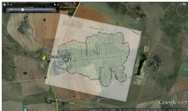
*Figure 1 Old underground mine plan adjacent to the Witkranz discharge point.*
