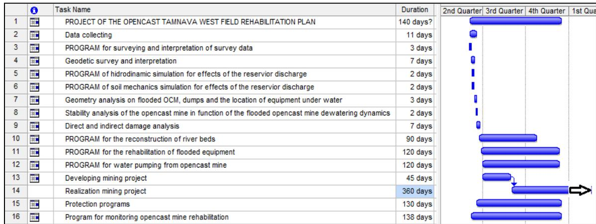
Figure 3 The opencast Tamnava-West Field dynamics of the project implementation.
