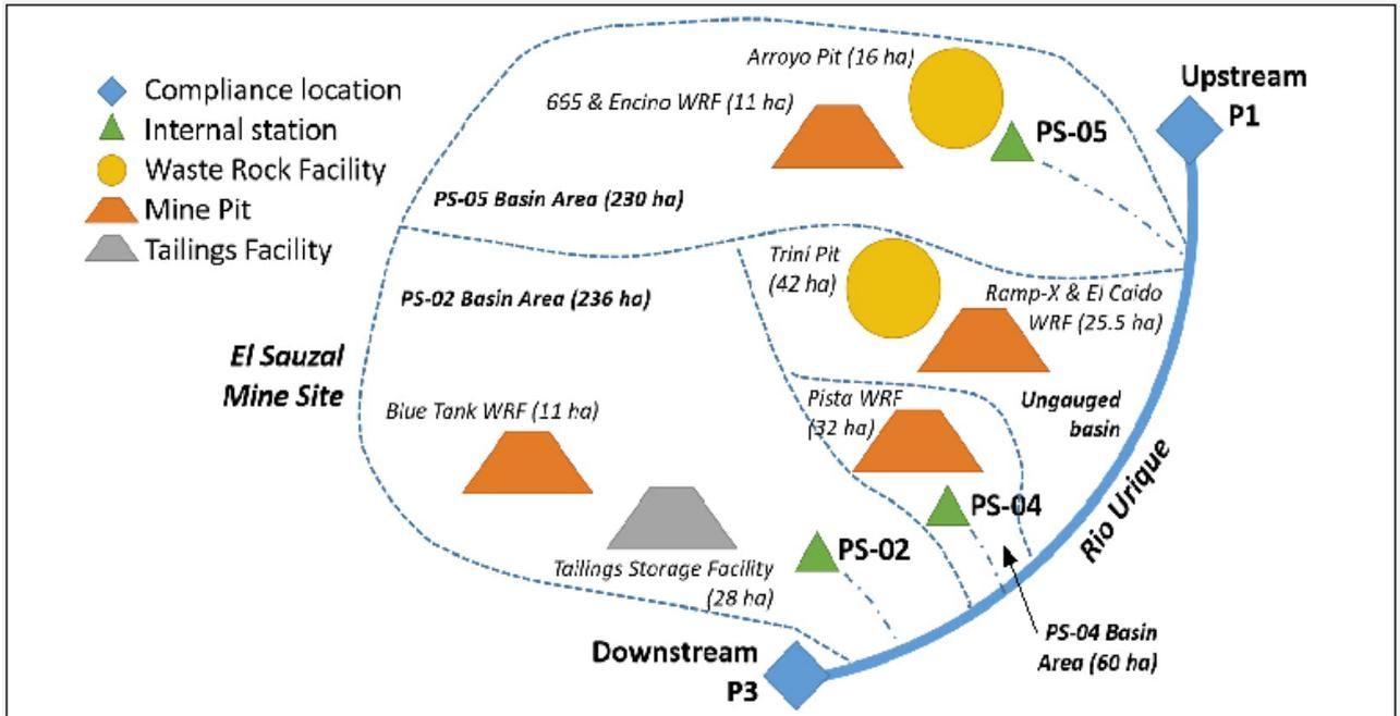
Figure 3: Schematic of El Sauzal mine site.
