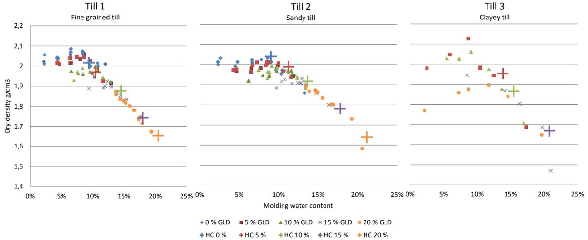
**Figure 2** Proctor compaction curves, with dry density ( $\text{g/cm}^3$ ) plotted towards molding water content of the different tills and till-GLD mixtures. The pure tills are plotted with blue rhombs, 5 w. % GLD-mixtures in red squares, 10 w. % GLD-mixtures in green triangles, 15 w. % GLD-mixtures in purple crosses and 20 w. % GLD-mixtures in orange dots. The plus-marks represent the estimated dry density and molding water content of the samples tested for hydraulic conductivity (HC).
