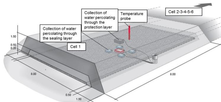
**Figure 1** The pilot cell at Boden, northern Sweden which consist of six different cells with a 0.5 m sealing layer and a 1.5 m thick protection layer on top of that. The sealing layer consist of till and 10 w. % of GLD from different paper mills. The protection layer consist of a fine grained till.
