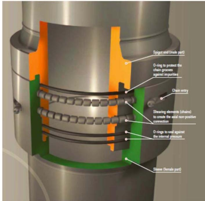
**Figure 2** ZSM Coupling for vertical free-hanging piping columns
