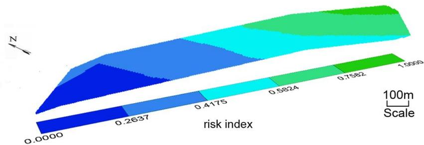
*Figure 5 Three-dimensional zoning for mining feasibility*
