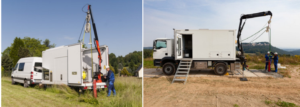
Figure 2 Trailer mounted deep pumping unit MTA-200 (left) and deep pumping unit MTP-350 (right) during sampling operations on deep groundwater monitoring wells at the Königstein site
