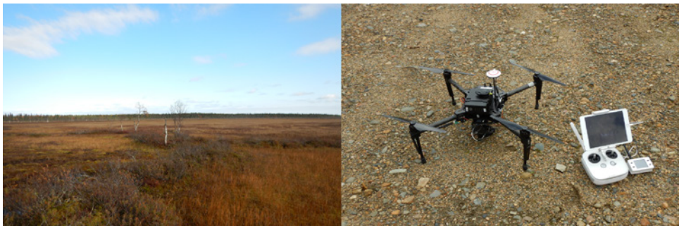
Figure 3 Viiankiaapa mire (on the left) and the UAV-TIR platform (Matrice 100) with TIR and RGB cameras (on the right).
