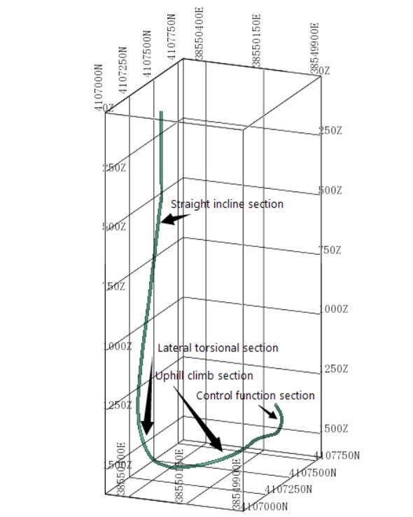
**Figure 1** 3-D directional well structure.
