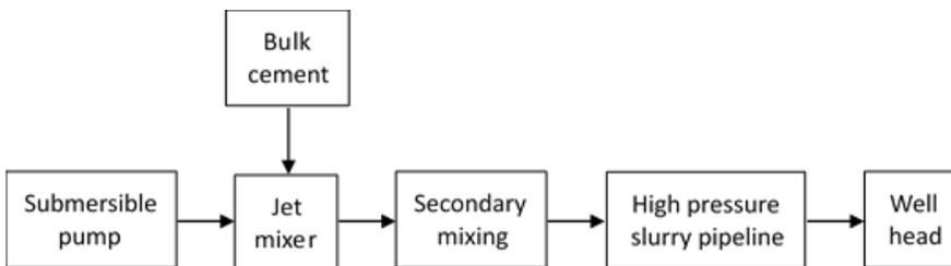
**Figure 3** Grouting process flow diagram.
