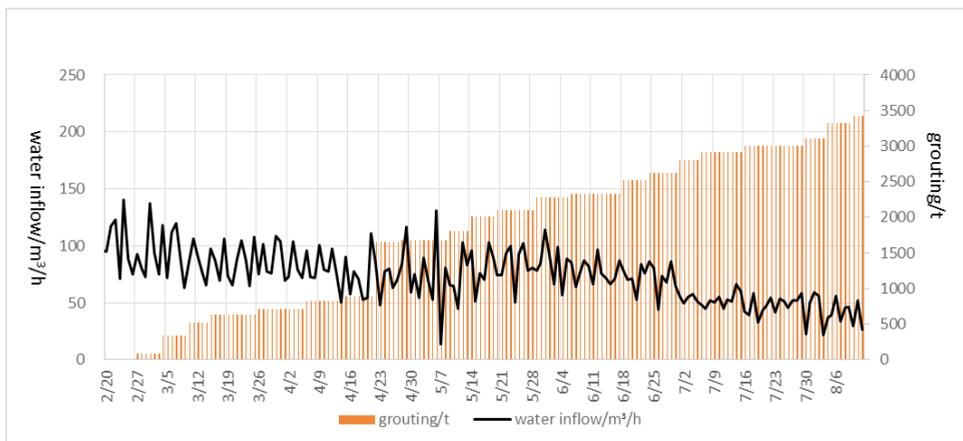
**Figure 5** Mine water reduction during grouting process
