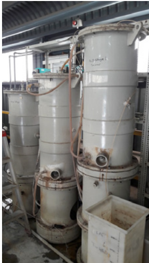
Figure 1 Multi-stage column system
