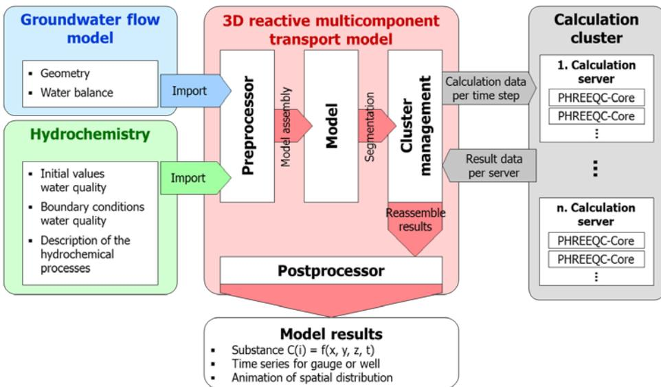
*Figure 2: Structural scheme of the reactive multicomponent transport model*
