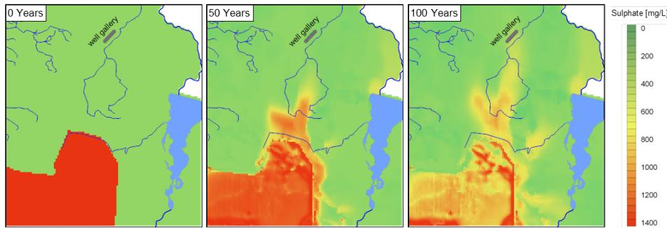
**Figure 4:** Distribution of the sulphate concentration in the 3rd aquifer of the multicomponent transport model at the start of simulation (left), after 50 years (middle) and after 100 years (right)
