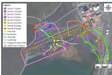
**Figure 10** – Survey Coverage and Summary of Detected Seepage and Drainage Paths for Main Dam Area
