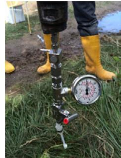
**Fig. 3** Outlet valve of the VS
