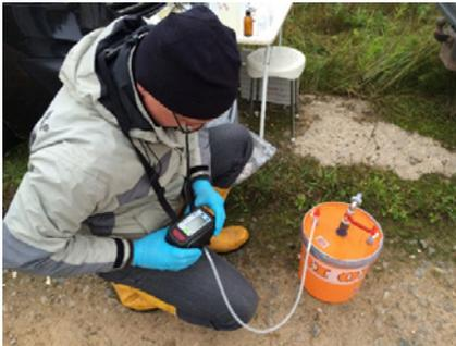
**Fig. 1** On-site Measurement of gas phases
