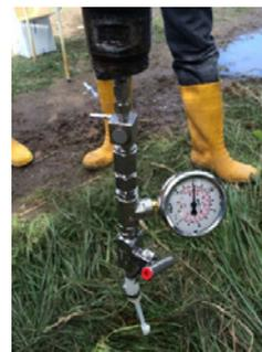
**Fig. 3** Outlet valve of the VS
