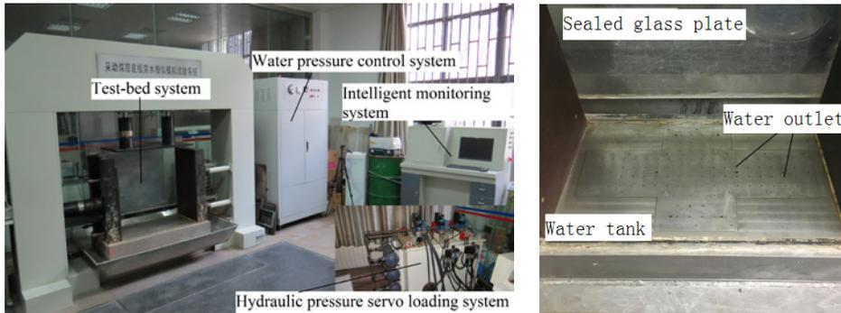
**Fig. 1** Similar Simulation Experiment System for Water-inrush From the Mining coal seam floor
