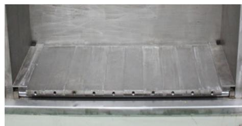
**Fig. 4** Coal seam drawing board
