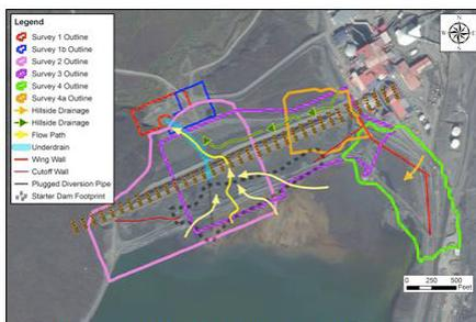
**Figure S1** – Survey Coverage and Summary of Detected Seepage and Drainage Paths for Main Dam Area
