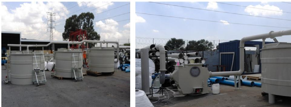
**Figure 4** Biological sulphate reduction pilot plant, showing the reactors (left) and the gas scrubber (right)
