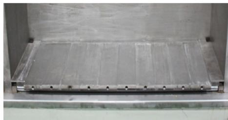
**Fig. 4** Coal seam drawing board
