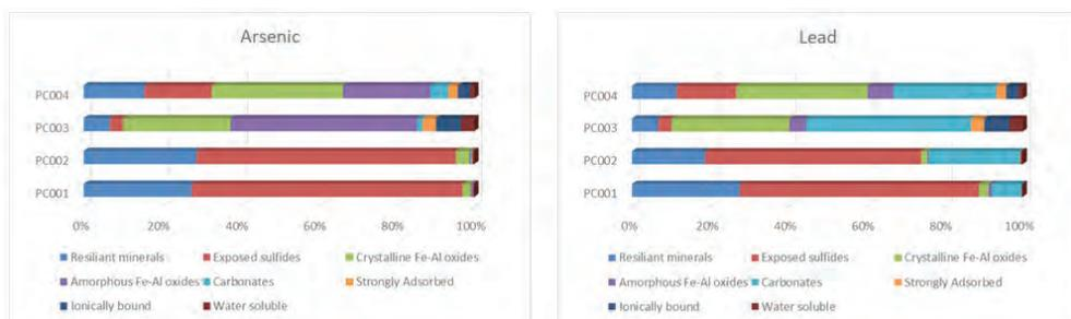
**Figure 1** Results of Selective Extraction Testwork for Arsenic and Lead
