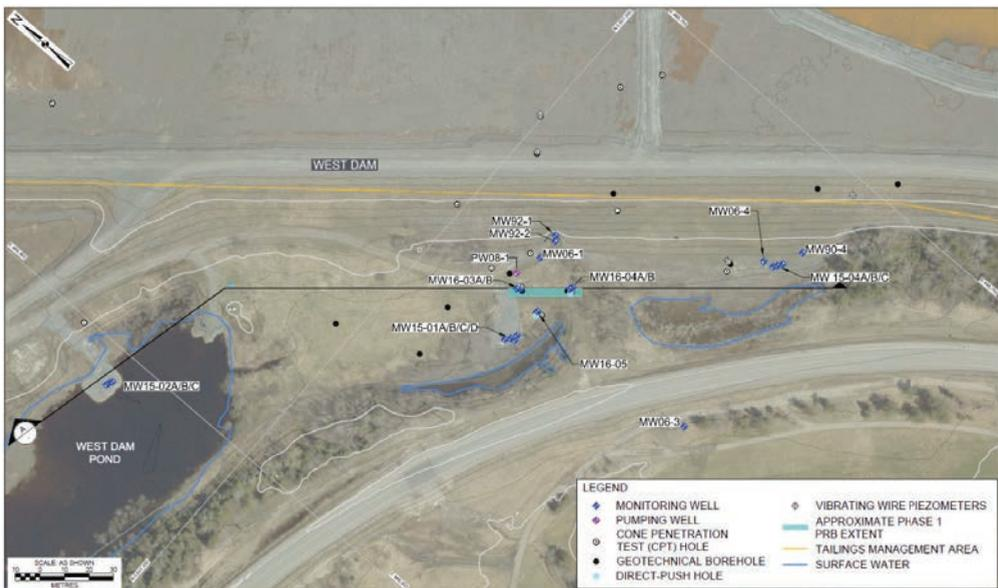
Figure 1. Location of proposed PRB, downstream toe of West Dam of the Campbell Complex TMA.
