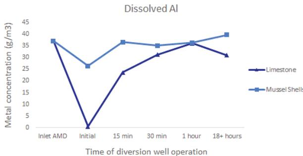
*Figure 4 Graph showing comparison of dissolved Al concentration for limestone and mussel shell treatment. Limestone shows greater decrease in concentrations, indicating it is more effective at treating AMD in a diversion well compared to the mussel shells.*
