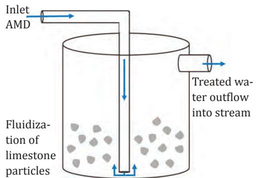
Figure 2 Schematic diagram of a diversion well.
