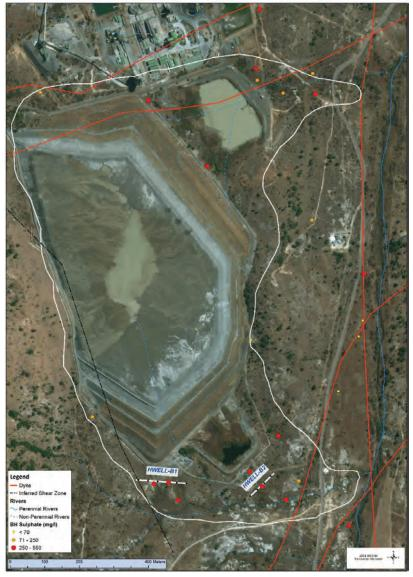
Figure 1 Simulated sulphate plume extent.
