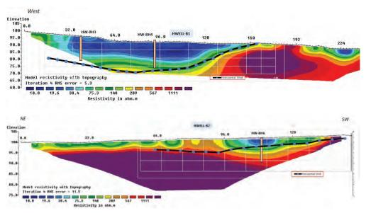
Figure 3 Horizontal borehole profiles in relation to the closest resistivity results.
