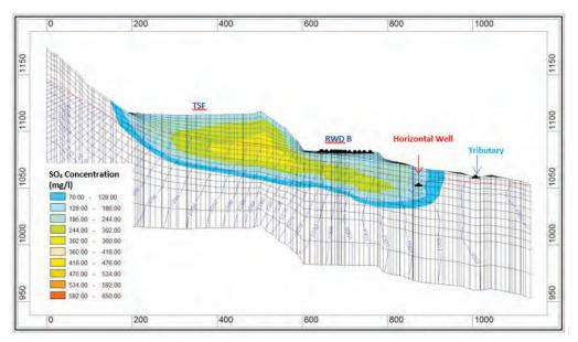
*Figure 5* Cross section showing simulated plume extent 15 years after hydraulic plume containment using horizontal boreholes commenced.
