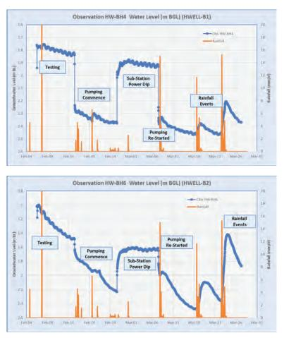
Figure 4 Drawdown results from longer term tests.
