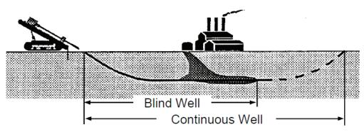
*Figure 2* Horizontal well used to intercept a plume. The solid line represents a blind well; the solid line plus the dashed line represents a continuous well. (EPA, 1994).
