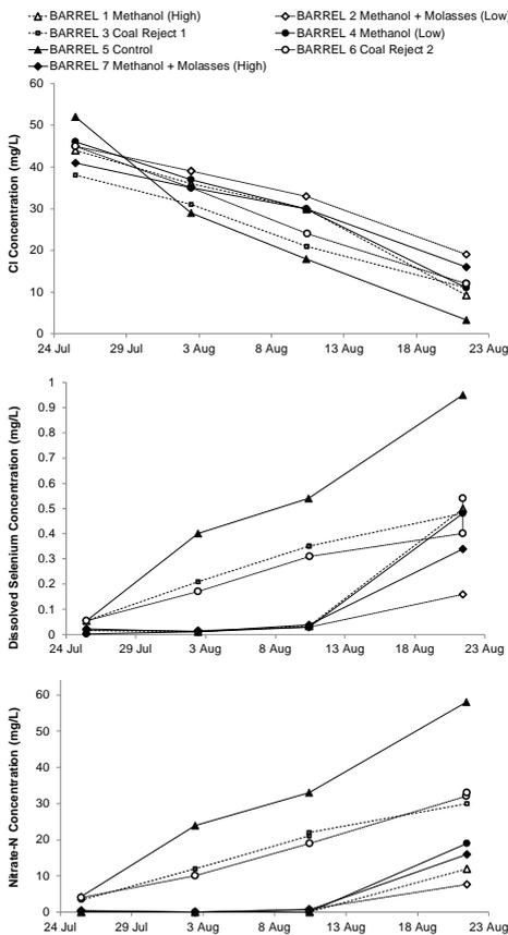
**Figure 2 Chloride, Diss. Selenium and Nitrate-N Concentrations in Test Barrel Effluent**
