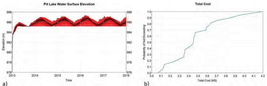
**Figure 4** Coupled model results a) probabilistic pit lake water surface elevation history b) total cost CDF.
