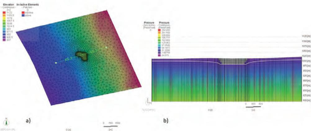
**Figure 3** Example FEFLOW open pit system groundwater model a) plan view b) Section XS-2.
