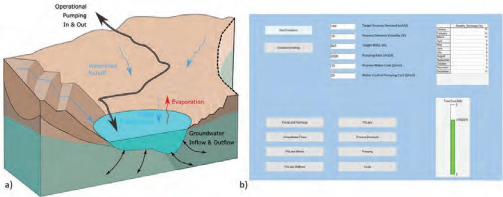
Figure 2 a) Pit lake water balance schematic and b) example application dashboard.
