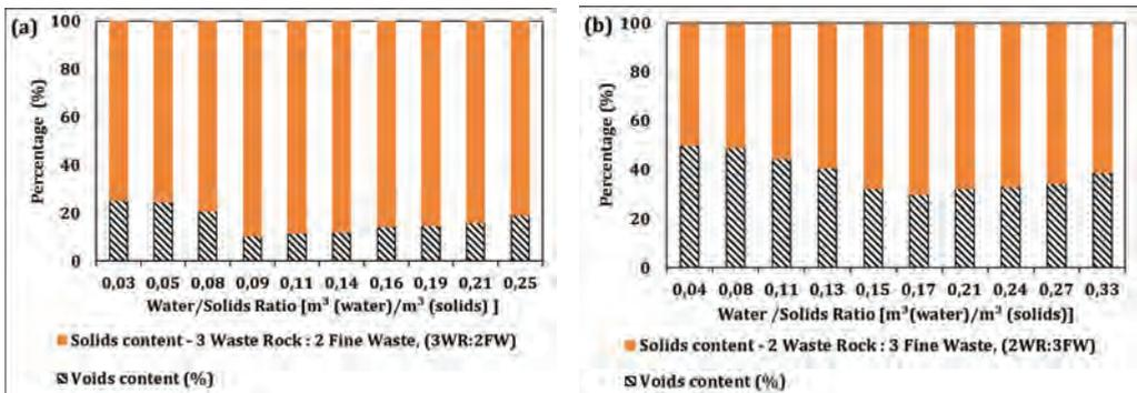
Figure 3 Relationship between solids and voids content for blends in dry mass ratio (a) 2WR:3FW (b) 3WR:2FW
