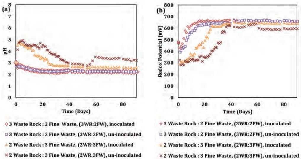
Figure 1 Biokinetic pH and redox potential profiles for tests performed on waste rock (WR) and fine waste (FW) blends
