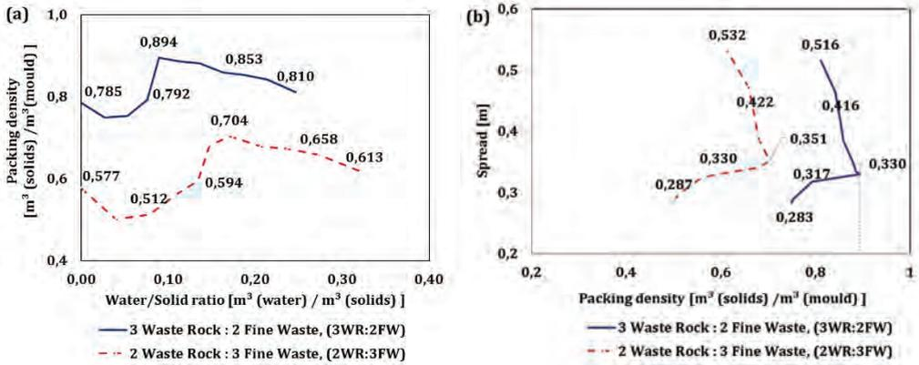
Figure 2 (a) The effect of water/solid (W/S) ratio on the solid concentration and (b) the relationship between packing density and spread
