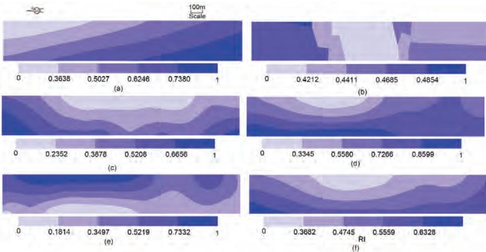
(a) water-yield property of the lower aquifers; (b) height of overburden failure; (c) overlying strata thickness; (d) thickness of the bottom clay layer of the Neogene system; (e) contour map of the elevation of bedrock surface; (f) risk index of the quicksand
