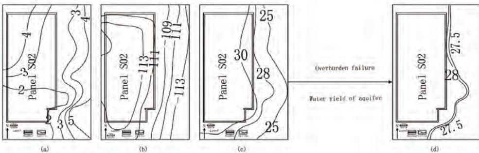
(a) isopach map of the bottom clay; (b) contour map of the elevation of bed rock surface; (c) isopach map of overburden; (d) the size of safety pillars under aquifers
