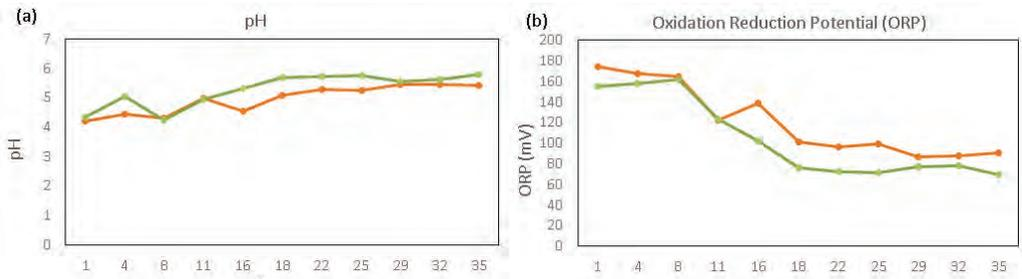
Figure 2 - Parameters measured in the five weeks of the experiment: a) pH and b) ORP
