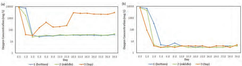
Figure 4 - Oxygen concentration in Column 2 (abiotic) with: a) normal range oxygen sensor (0-100% or 0-45mg/L) and b) low range oxygen sensor (0-5% or 0-2 mg/L) on a log scale with base 10 (Y-Axis)
