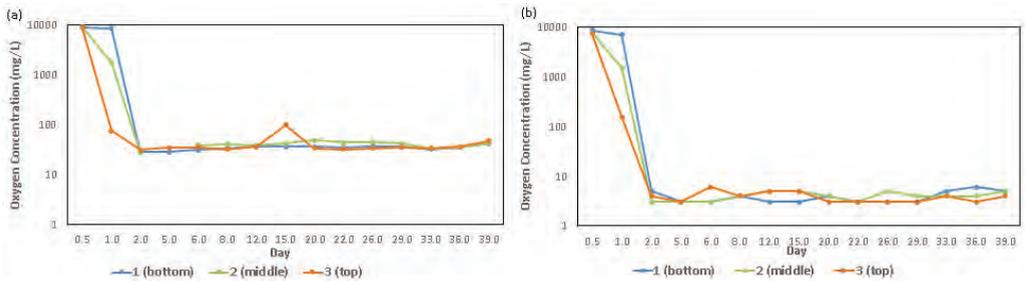
Figure 3 - Oxygen concentration in Column 1 (biotic) with: a) normal range oxygen sensor (0-100% or 0-45mg/L) and b) low range oxygen sensor (0-5% or 0-2 mg/L) on a log scale with base 10 (Y-Axis)
