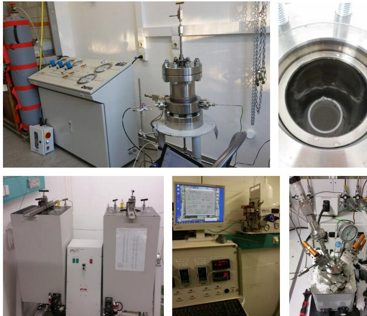
**Figure 1** Autoclave systems used in the experiments. Top pictures show autoclave 1, Bottom left and center show autoclave 2 and bottom right shows autoclave 3.
