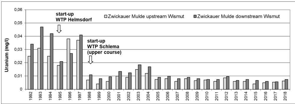
Figure 3 Uranium concentrations (median) in surface water of Zwickauer Mulde upstream and downstream of remediation site Crossen-Helmsdorf
