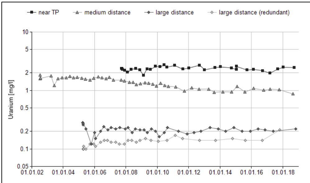
Figure 2 Uranium concentrations in groundwater along Wüster Grund disturbance (permian) in dependence of distance to TMF Helmsdorf
