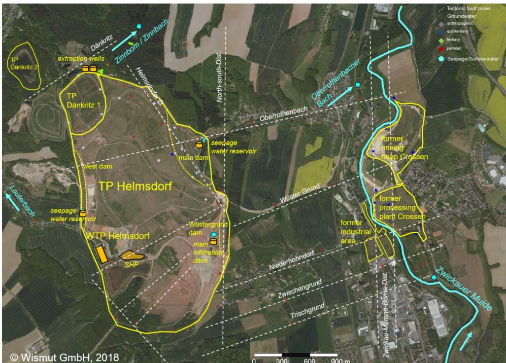
**Figure 1** Overview of the Crossen-Helmsdorf site including the most important objects, water catchments, schematized tectonic fault zones and points of key monitoring network 2018
