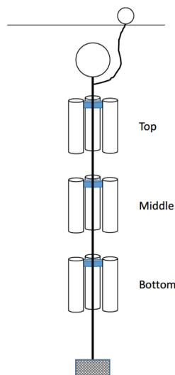
Figure 2 Diagram of the arrangement of the sediment traps used in the lakes
